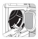
Your dryer will only function well if the filters are clean. The filters collect all the fluff which accumulates during drying and they must therefore be cleaned at the end of each programme, before removing the laundry, with a damp cloth. The filter light is on to remind you of this operation.
